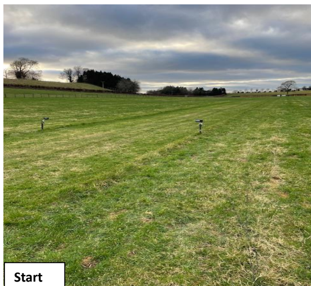
Plate 6: Built in timing system with beams placed on the gallop, one set at take-off (start) and one set when slowing down (finish) to accurately start the time of each subject's performance – (authors own 2024).
