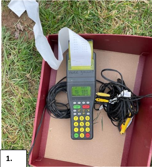
Plate 7: (1) Handheld timing device which automatically prints off times of each subject once passed the second set of beams and (2) Lure used throughout data collection – (authors own, 2024).
