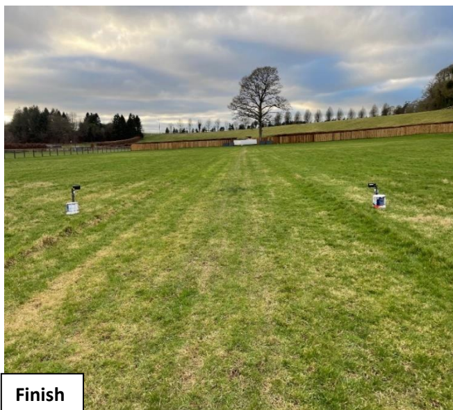
Plate 6: Built in timing system with beams placed on the gallop, one set at take-off (start) and one set when slowing down (finish) to accurately start the time of each subject's performance – (authors own 2024).
